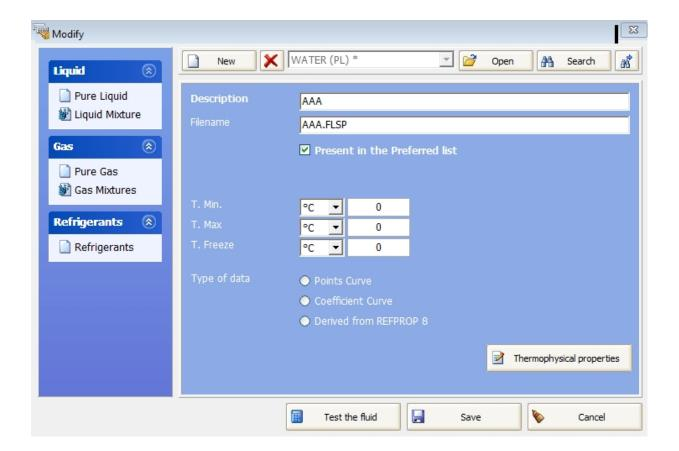
•Here you can insert the minimum and maximum temperature of validity of the fluid, the freeze temperature and the type of data that describe the fluid. Clicking on the button the type of data that describe the fluid. Clicking on the button the type of data selected before:
