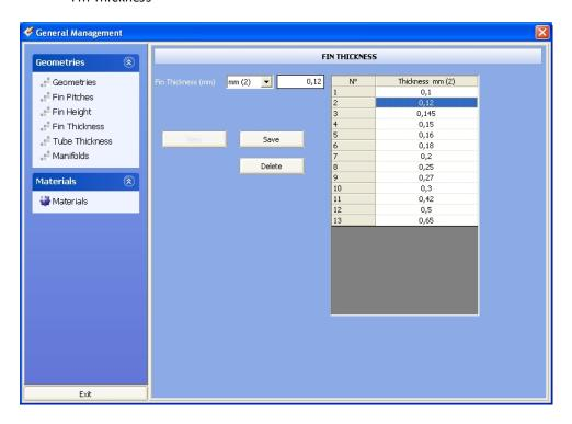
Here again to add a new Thickness to see in the main program, we have to insert the value in the Fin Thickness box, then click on the "New" button
