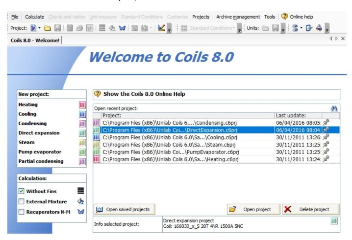
We can open new project by clicking on the left part like Heating, Cooling, Condensing, Direct expansion, Steam, Pump Evaporator and Partial condensing.
