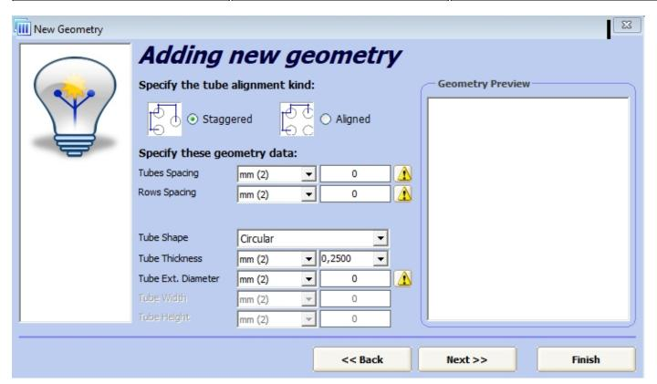
• Let's leave the tube alignment "Staggered" and click on the "Next" button after enter 7 mm as external diameter, 19,05 mm as tube thickness, 16,5 mm as rows spacing,
