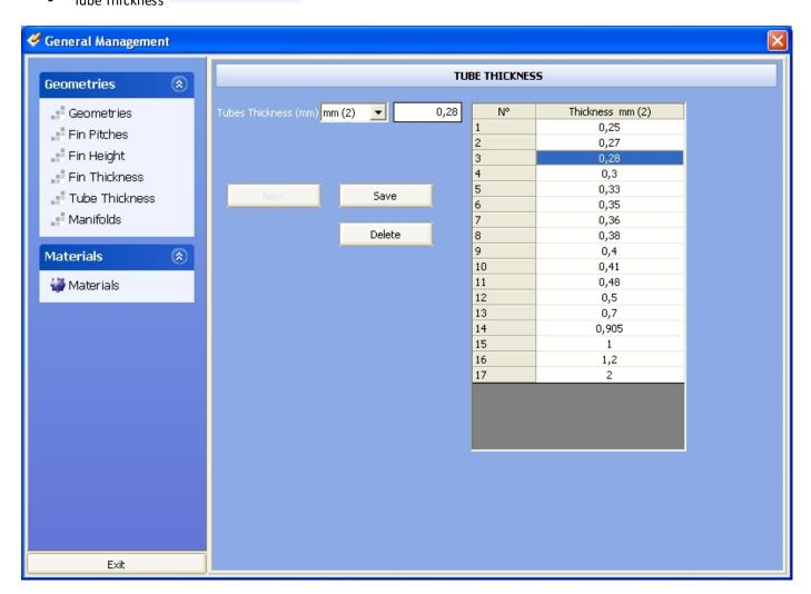
Here again to add a new Thickness to see in the main program , we have to insert the value in the Tubes
