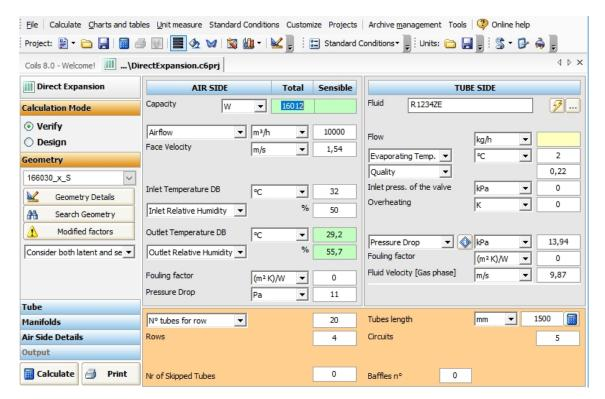
We can see, that in the bottom part of the calculation form we do not mention the fin, because the tube is smooth or bare
