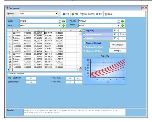
Then click on "Save" and "Back", you will see the capacity, current and absorbed power curves in the main mask:
