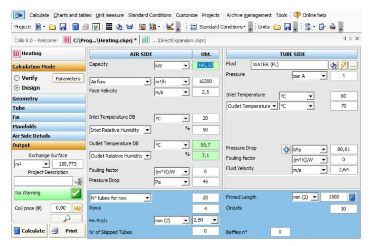
where on "Air Side" we can see "Pressure Drop" measured in Pa, as calculation's result.
