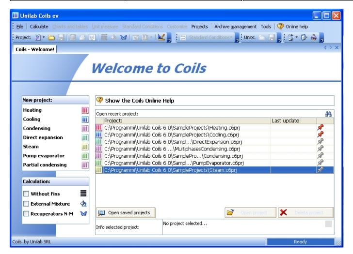
Under the New Project, We have the possible calculation modes the battery.
