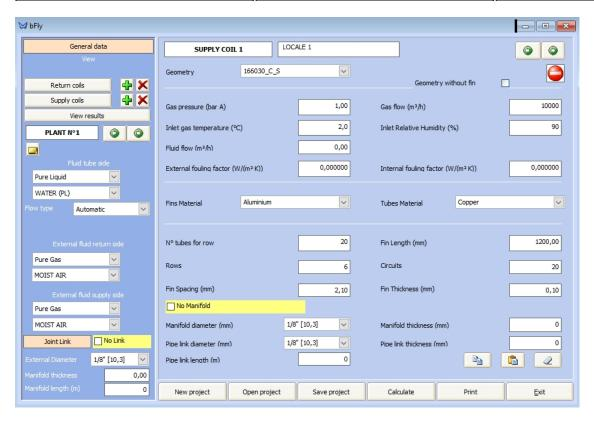
This is an example of the supply coil. As you can see, in the data inserted, the supply coil has lower inlet temperature, than the return.
