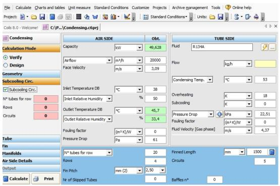
Then we can insert the data relative to the subcooling part, which are: "N° tubes for row", "Rows" and the "Circuits", which are the input values, as we can see in the following screen.
