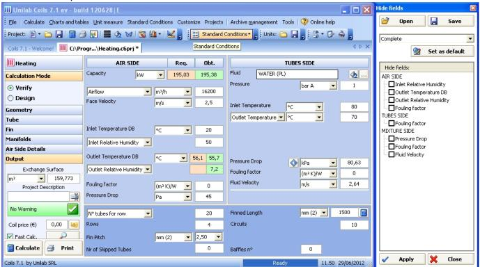
You can select the fields you want to hide for the particular mode of the coil (heating, cooling, etc.) and save this setting to open it in a future calculation.
