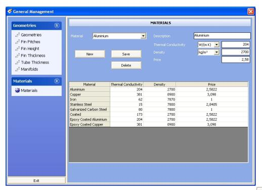
Here we can manage the data of the materials to use in the main program. With the button you can insert a new material and the relative data.
