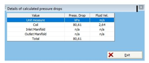
We hit the "Design" button and obtain the following, where you should set the tolerances and the required capacity
