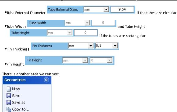
This allows us to copy the geometry in other calculation modality, if we need it, after hitting the "Copy to..." button.
