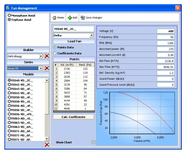
Here you can modify the data of the fans already inserted in the archive, insert a new one by the button , o delete a model selected in the left list:
