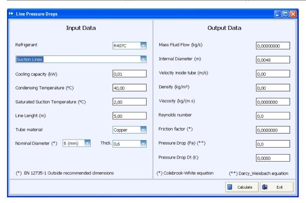
Where we can calculate the pressure drop for a specific refrigerant along the suction, discharge and liquid lines.
