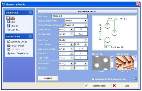
In the next screen we have two types of Coils, spiroidal and integral. We choose the integral one
