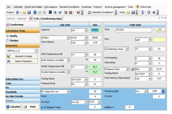
This refers to a coils without subcooling circuit. To do its calculation, we can click on the "Subcooling Circ."
