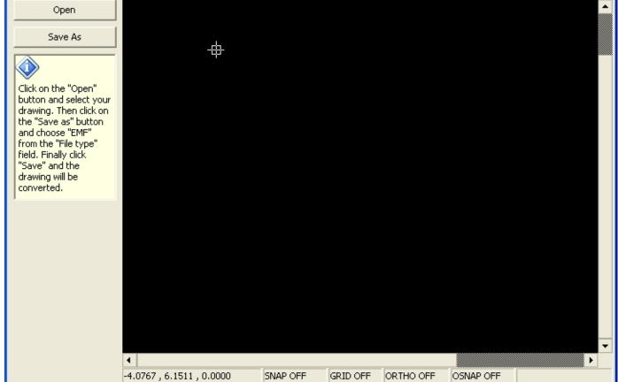
Open Save As Here you can open a DXF / DWG file by and save it into an EMF file by
