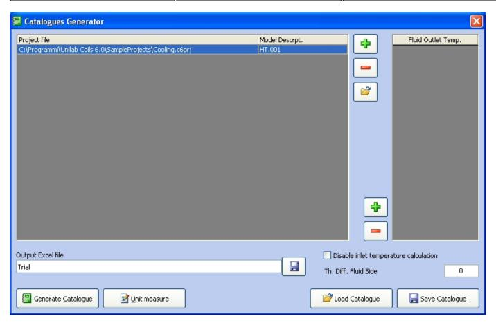
In the grid at the top right hand side we insert the temperature fluid, which will vary will be included in the columns of the Excel sheet. These temperatures vary depending on the mode of calculation:
