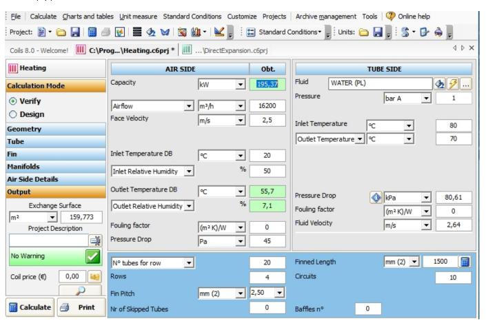
where the "Capacity air Side" is calculated
