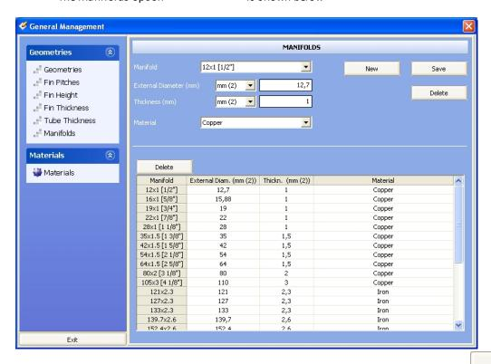
Here we can manage the data of the manifolds to use in the main program. With the button manifold and the relative data.
